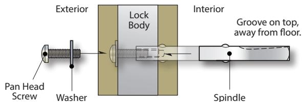
4. From the exterior side of the door, measure the distance to the middle of the lock body. Cut the thumb piece stem to this length.
