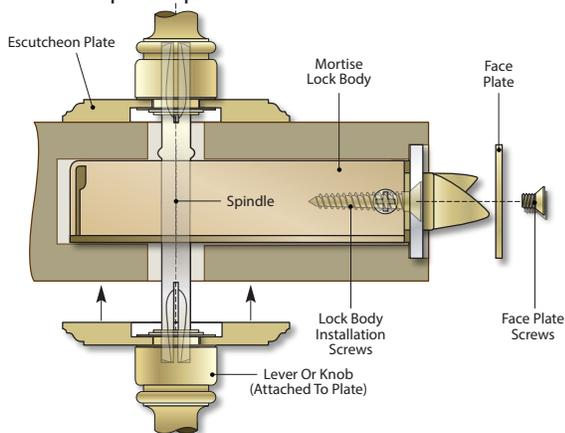
Next align the interior plate so the spindle engages the lever. Adjust the plates to sit square with the door edges.
