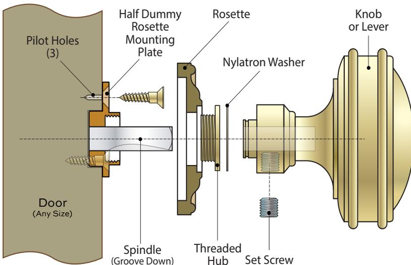
6. Slide the knob or lever over the spindle and press until it seats firmly against the rosette. The nylatron washer is not required for this application, but may minimize any gapping between the knob or lever and the rosette.
