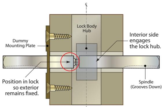
**Note:** For this application, it may be necessary to remove the security notches located on the spindle.
