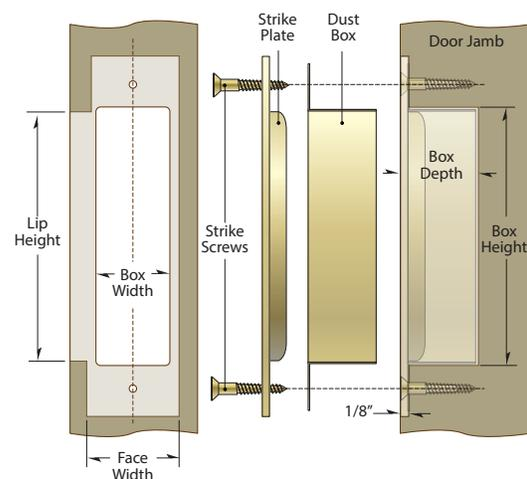
Finally, mortise the jamb to the proper depth to accept the dust box.
