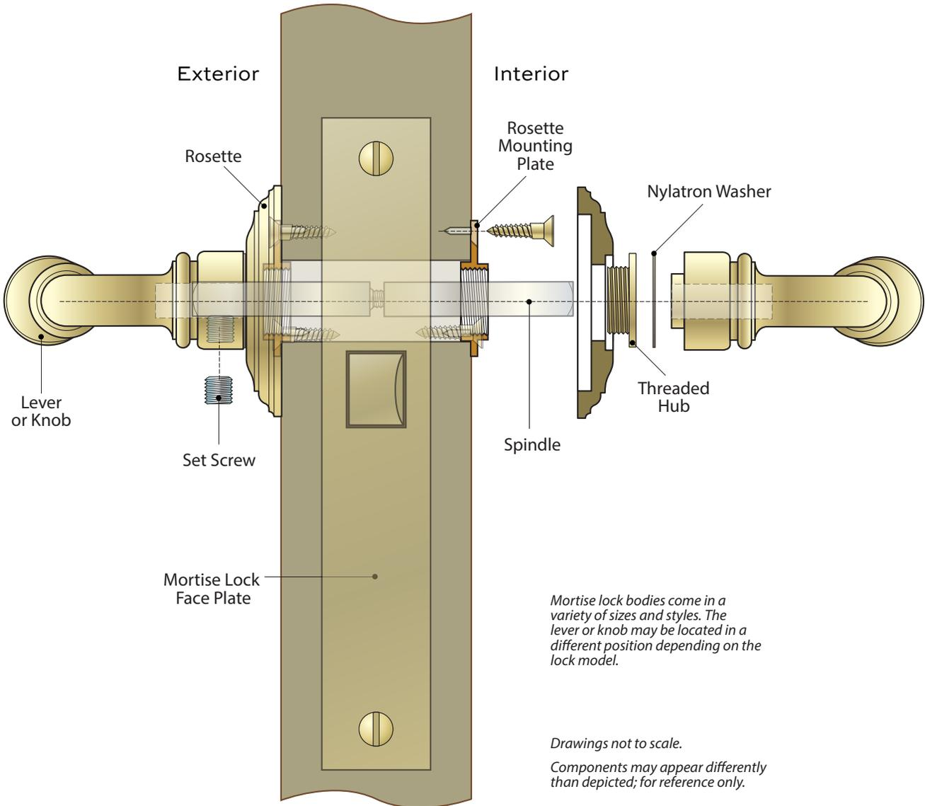
*Mortise lock bodies come in a variety of sizes and styles. The lever or knob may be located in a different position depending on the lock model.*
