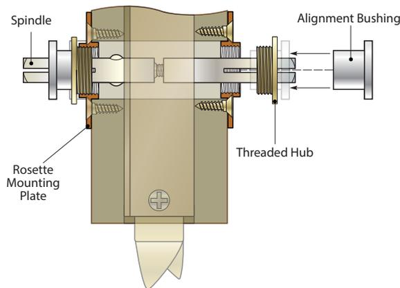
5. Position a rosette mounting plate with a threaded hub on both sides of the door. Insert the two alignment bushings into the hubs and snug the mounting plates firmly against the door surface.
