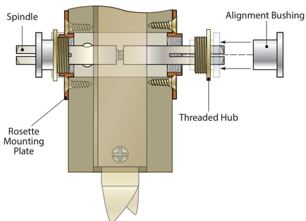
6. When satisfied that the spindle is level and aligned, mark the screw hole locations for the rosette mounting plates. Drill pilot holes and proceed to affix the plates to the door surface with the screws provided.
