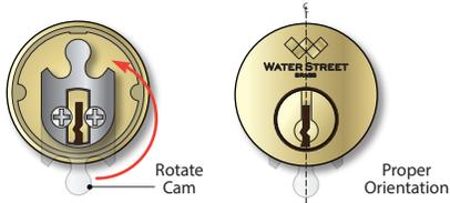
Make sure the cylinder is properly oriented as shown. Secure the cylinder by tightening the cylinder retention screw found inside the lock body. Test the function of the lock cylinder.
