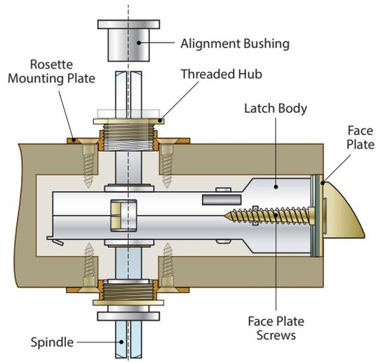
5. Insert the spindle through the latch body as shown. Position a rosette mounting plate with a threaded hub on both sides of the door. Insert the two alignment bushings into the hubs and snug the mounting plates firmly against the door surface.
