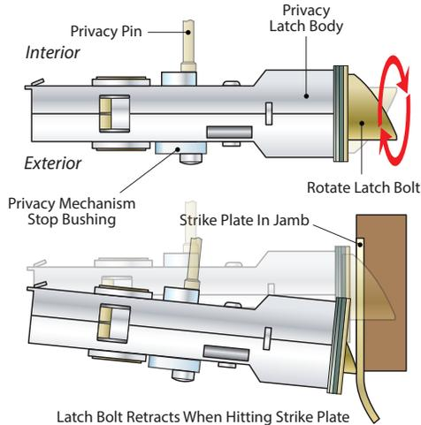
4. Install the latch body and face plate into the door and secure loosely with the screws provided. Do not tighten completely at this time.
