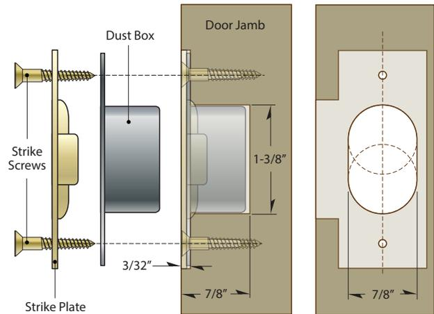
After installation, if the latch does not fully engage with the strike, loosen the screws and adjust slightly.
