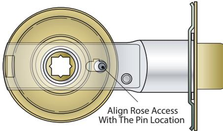
in the rosettes to sit directly in line with the privacy mechanism in the latch. Firmly secure the threaded hubs using the tool provided. Take care not to scratch or mar the rosette surfaces when installing.
