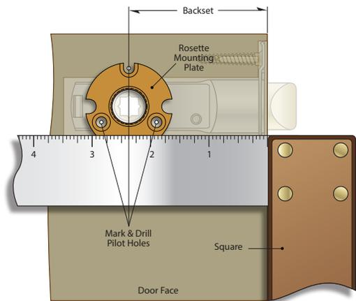
6. Tighten the latch face plate screws. When satisfied that the latch is firmly in place and level, mark the screw hole locations for the rosette mounting plates. Drill pilot holes and attach the plates to the door surface with the screws provided.
