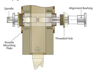
6. When satisfied that the spindle is level and aligned, mark the screw hole locations for the rosette mounting plates. Drill pilot holes and proceed to affix the plates to the door surface with the screws provided.
