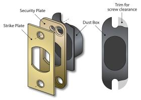
16. Finally, install the strike plate over top of the security plate, using the finished strike screws as shown.
