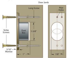
14. Mortise the dust box cavity as shown. Position the security plate in the jamb and mark the screw hole locations. Drill 1/8" diameter pilot holes for the screws.
