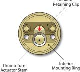
11. Position the interior mounting ring assembly into the interior plate. The cylinder tailpiece will slide into the back of the thumb turn actuator. Install the two machine screws into the cylinder mounting attachments and tighten firmly.
