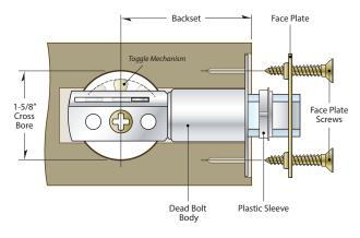
Before installing the two deadbolt cylinders, slide the provided deadbolt bracket through the bolt body as shown on the assembly drawing. The legs should protrude from the interior side towards the exterior.
