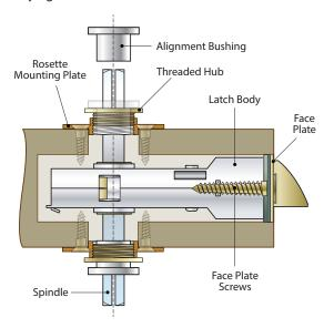
5. Tighten the latch face plate screws. When satisfied that the latch is firmly in place and level, mark the screw hole locations for the rosette mounting plates. Drill pilot holes and proceed to affix the plates to the door surface with the screws provided.
