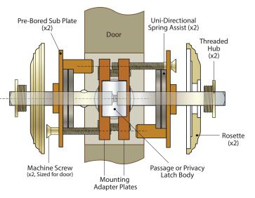
Since these spring assist mechanisms are unidirectional, it is important to double check the direction of the spindle rotation. The levers should operate the latch by pushing down, as shown here.
